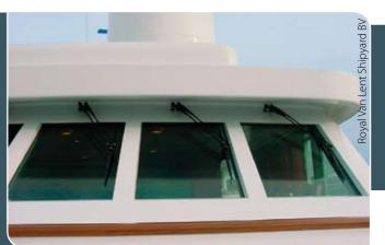
The size and shape of the glass that has to be wiped determines which motor, arm and blade is needed. The larger the wiping area, the larger arms and blades have to be to cover the area. And the larger the arms and blades are, the stronger the motor has to be.
